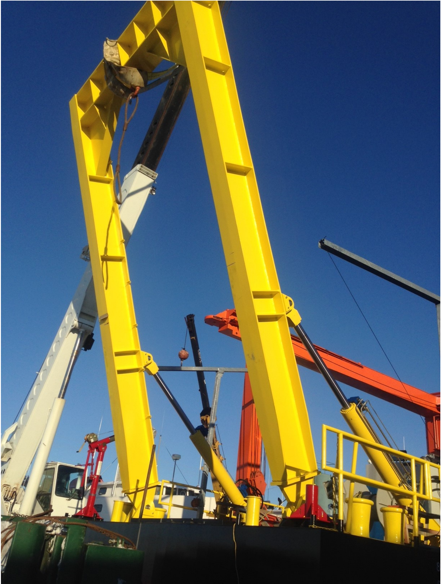
Hydraulic cylinders utilized to operate an A-Frame system on a research vessel utilized on the West Coast of Canada.
