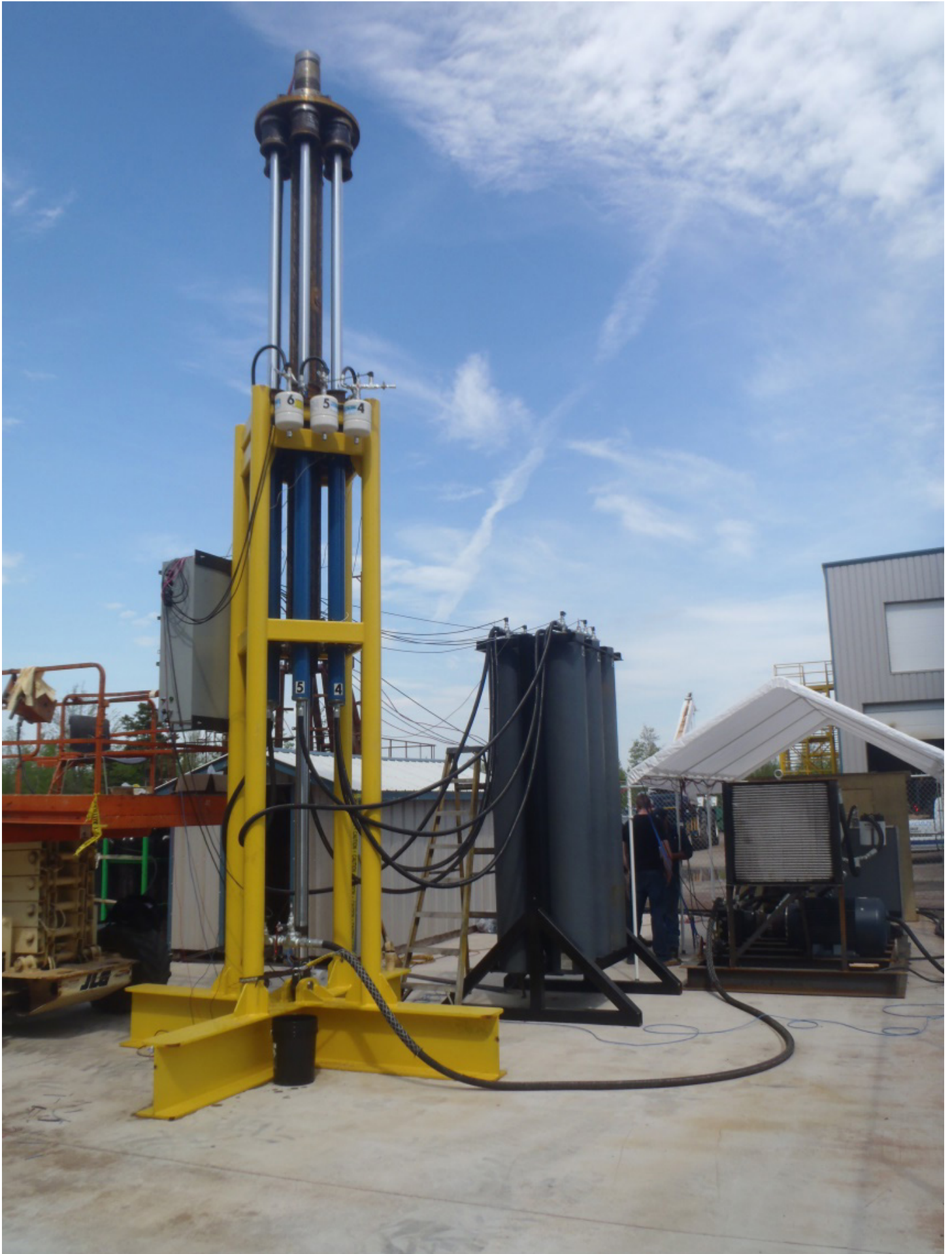
Development of a 1/5 scale prototype of a Tensioner System for operation in deep and ultra-deep water, designed / developed / load tested at our facility in 2014. The next phase of the project is the
